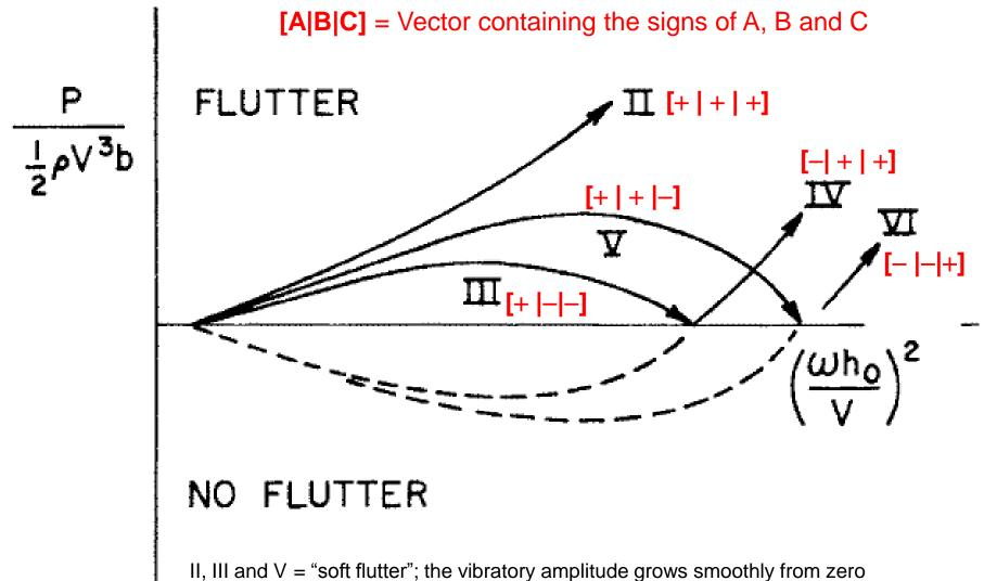
IV and VI = "hard flutter"; when flutter appears, the amplitude is a large finite value
